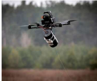
Tried and tested: A Ukrainian made FPV fibre-optic drone is displayed at a military market place in Kyiv, Ukraine. AP
